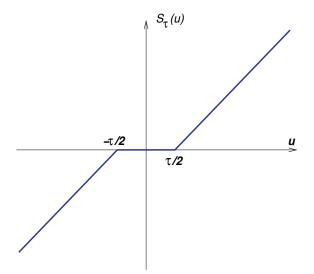
Figure 3: A plot of the soft-thresholding function  $S_{\tau}$ . The soft-thresholding operator shrinks the size of the components of its input vector in a continuous fashion.
